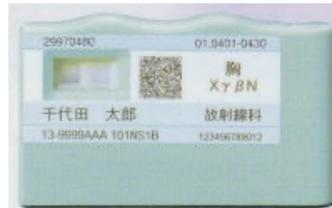
$\text{Ag}^+$ -activated Phosphate Glass + radiation  $\rightarrow$  (UV)  $\rightarrow$  fluorescence
