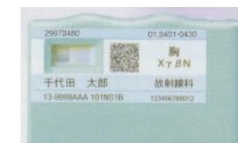
$\text{Ag}^+$ -activated Phosphate Glass + radiation  $\rightarrow$  (UV)  $\rightarrow$  fluorescence
